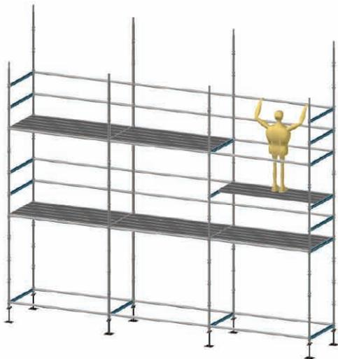
**Figure 4: Diagrammatic illustration of erection and dismantling using platform option for a five plank wide scaffold. Note: scaffold is shown against an existing building, so guardrails only needed on external face. Toeboards and lower mid-rails omitted for clarity.**
